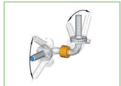
Swivel movement on both sides with type 13F in angled pipe piece
