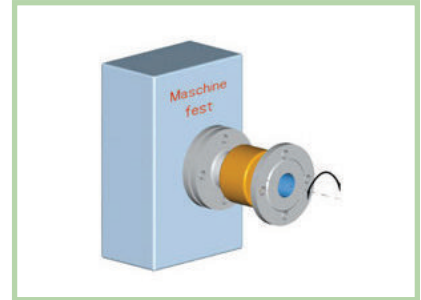
Slow rotary movement with type 11F (1 fixed point, 1 side flexible)
