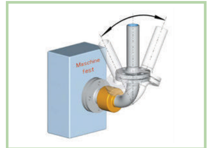
Swivel movement with type 12F (1 fixed point, 1 side flexible)
