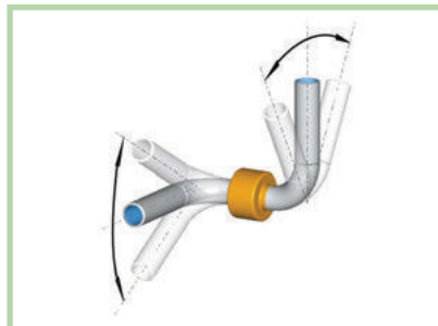
Swivel movement on both sides with type 13S in angled pipe piece
