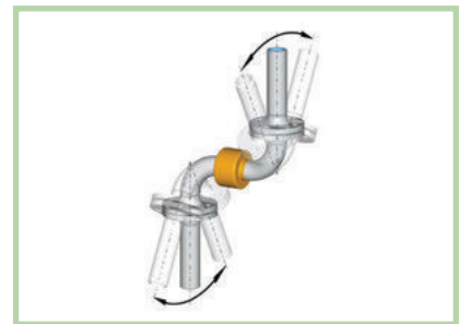
Swivel movement on both sides with type 13F in straight pipe piece
